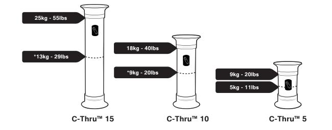
\*Glasdon recommends that the C-Thru 15 and C-Thru 10 are not filled beyond the mid-point of the body to improve handling and extend the lifetime of the product.
